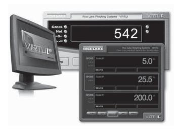
VIRTUi is a Windows\*-based desktop application that works with iQUBE\*/iQUBE² to replicate the IQ plus\* 355 indicator Ideal for system integrators and OEMs wanting toxinate a PC-based solution, VI RTUi provides the functionality of a basic weight indicator. Load cells are individually monital and calibrated, making setup easy
