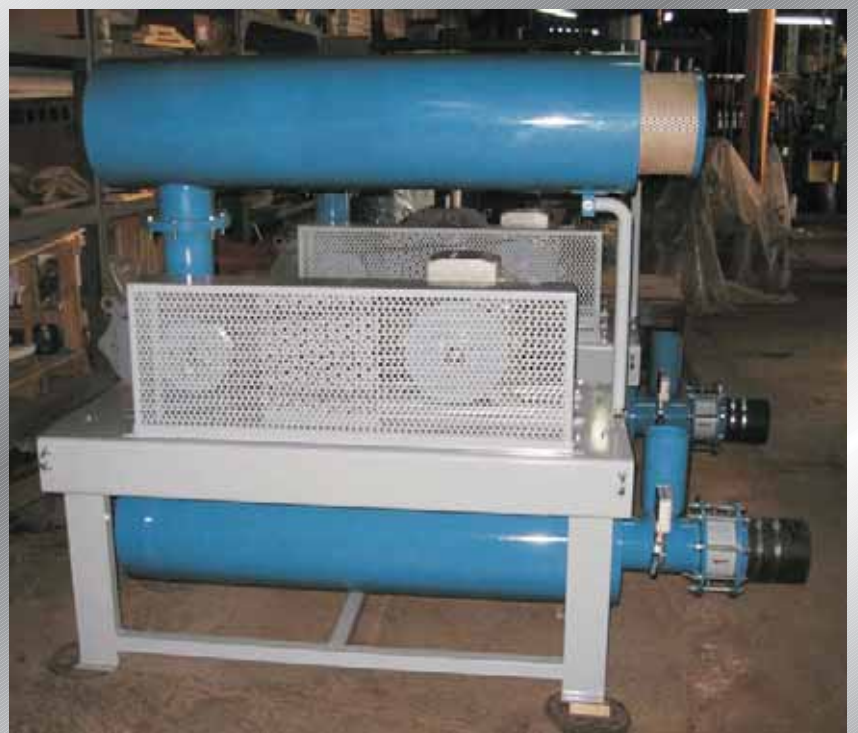
Blower set with silencer(front view)
