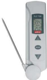
The TLC 720, Handheld Infrared Thermometers function as non-contact infrared and contact thermometers. The user can always toggle between the thermometer's two operating modes. Additionally the unit has a laser point that helps the user aim it at the target when making measurements.
